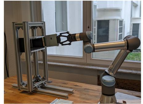
Figure 1: In our task, the robot has to insert a hard drive into a rack mount. Here, the challenge lies in the low clearance of the mount which requires highly precise motion based on force feedback to avoid jamming the disk. The task has to be solved based on demonstrations from a human expert, and we will consider a simulated version and the real setup.
