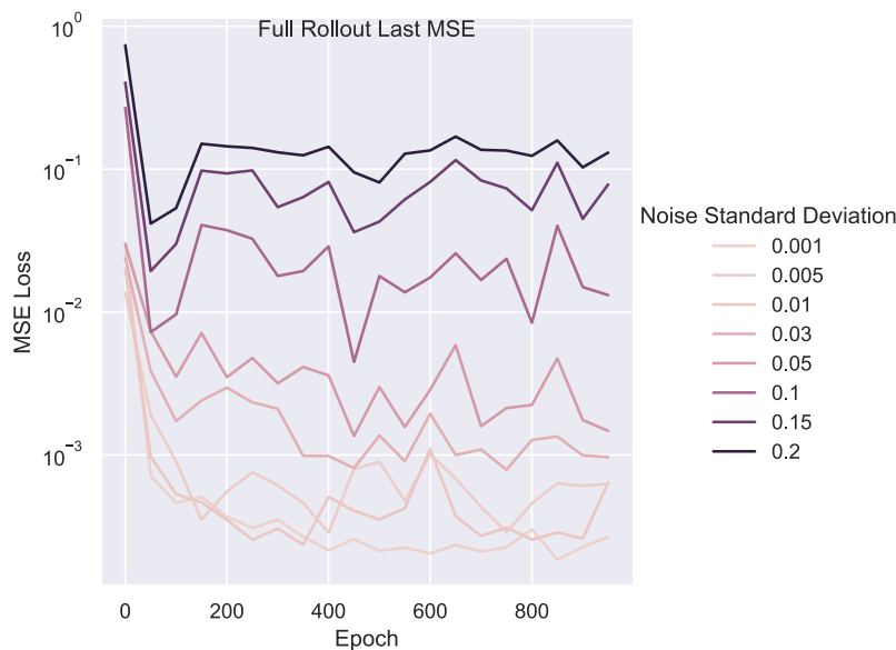
Figure 6.1: Evaluation of Rollout Stability of Simulators Trained with Different Noise variances
